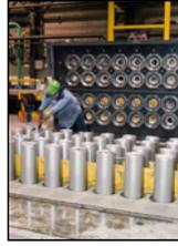
**COVER:** Before billets are removed from the Wagstaff casting pit at Sapa's Cressona, Pennsylvania facility, the chief caster stencils the cast order number onto the cast log. Sapa has made significant investments to increase their casting capacity.
