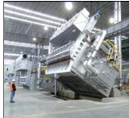
**COVER:** First tilting test of one of the 40 tonne tilting combination melting/holding furnaces installed by GNA alutech at Aluminicaste in Mexico.
